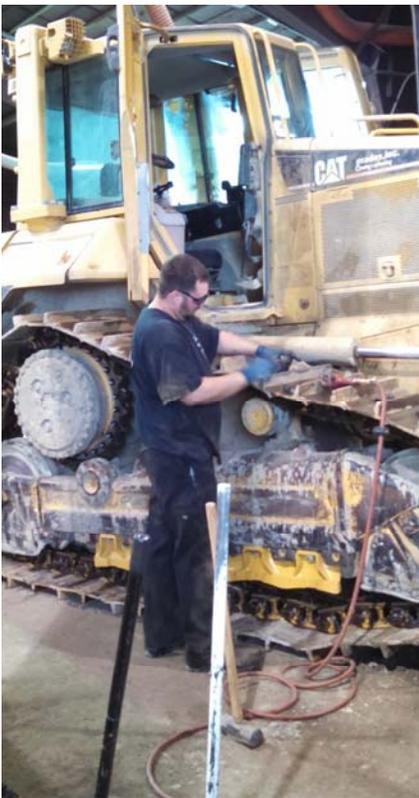
Chaz Baledge installing tracks on a D6N at the shop.
